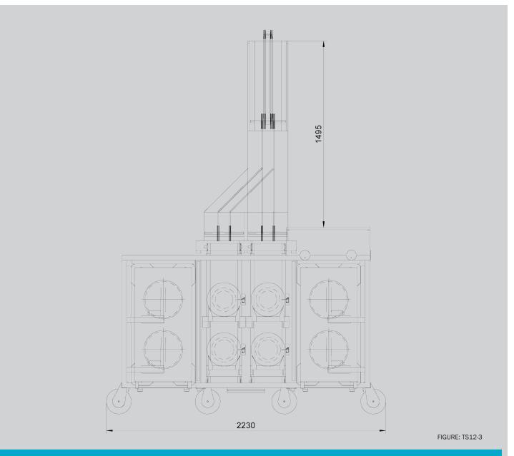
The plate stacking unit TS12-3 for stacking two different plates by type into two double plate dispensers with the automatic discharge of the dispenser trolleys.
